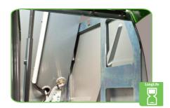
The chassis is completely galvanised and offers therefore the best corrosion protection for the welded constructions made of steel.
