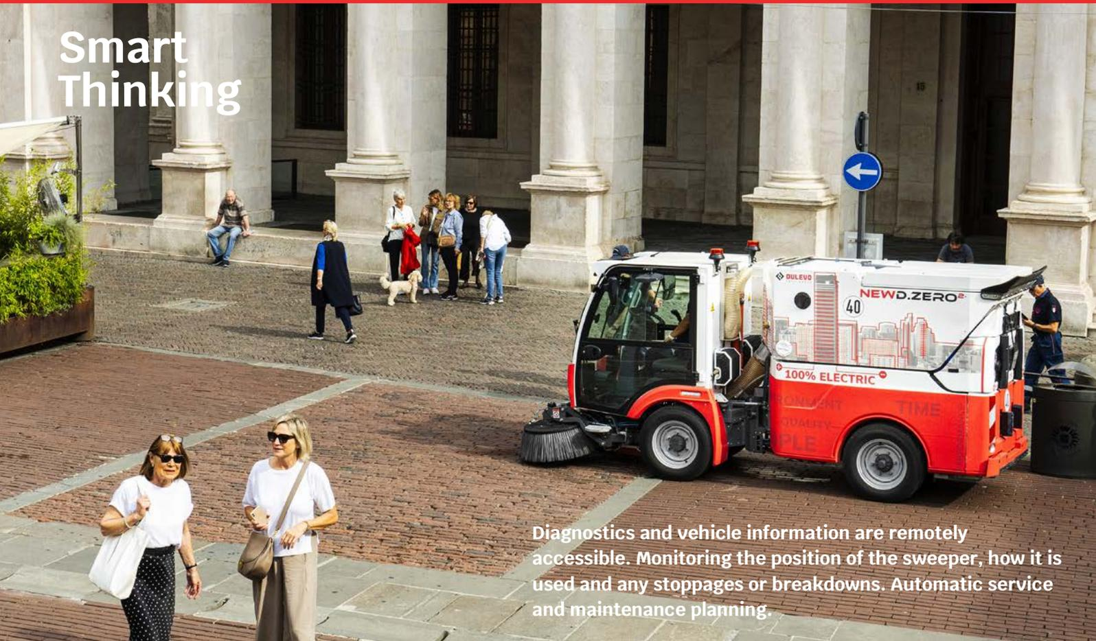
Diagnostics and vehicle information are remotely accessible. Monitoring the position of the sweeper, how it is used and any stoppages or breakdowns. Automatic service and maintenance planning.
