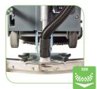
Squeege made of stainless steel with quick change release for replacing squeegee blades.
