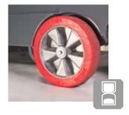
High driving comfort due to large dimensioned traction wheels with anti-slip and non-marking PU wheel tyres
