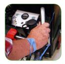
Steering handle made of stainless steel and wrist connecting to ground for the operator.
