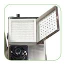
The exhaust air filter Hepatex MDH3A (option) matches filter class H 13 as to DIN EN 1822 with a maximum transmittance of 0,05 % (see also data sheet EURO-suspension Filter).
