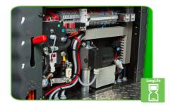
The ACX control enables the linking-up of different functions. In this way it controls optimally the operating status like the soft start of brush and suction motor, the GWS-control as well as all programmable parameter like braking performance and speed.
