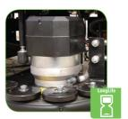
2 brushes guarantee efficient cleaning power. Swinging brush head to avoid impact damages
