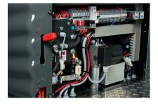
The ACX control enables the linking-up of different functions. In this way it controls optimally the operating status like the soft start of brush and suction motor, the GWS-control as well as all programmable parameter like braking performance and speed
